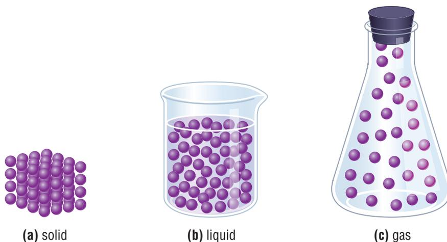
**Figure 3** (a) Particles of a solid are tightly packed and locked in place. (b) Particles of a liquid are freer to move about. (c) Gas particles have large spaces between them and are free to spread out to fill their container.
